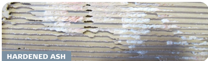
Hardened ash remaining in a DPF after a Bake'n'Blow cleaning.
